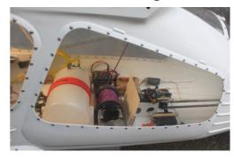
To prevent the towing lines from getting caught in an obstacle on landing, they are either dropped during a low-altitude fly-by or retracted using a winch installed in the fuselage. Only slow towing planes may be used for towing vintage gliders. Older aeroplane types such as the Piper are best.
