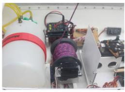
Winch to retract the towing line built in the fuselage
